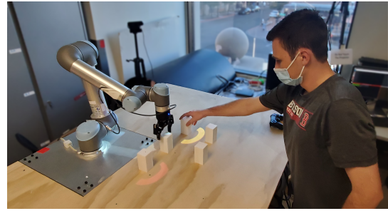
Figure 3: Highlight Mode: A user collaborating with the robot while information about the next object explicitly provided via projections in the form of semi-elliptical disc.
