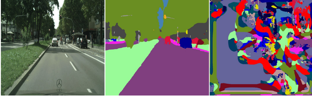
Figure 1: From left to right: the original image, the result under a stealthy attack, and the result under a non-stealthy attack.
