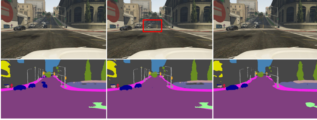
Figure 3: The three key steps of our proposed method. The first column displays the original image alongside its semantic segmentation results. The second column presents the inpainted image and its corresponding segmentation output, generated by masking and inpainting the central vehicle region. The third column shows the perturbation overlaid adversarial image and its segmentation results, illustrating the effect of the optimized perturbation.
