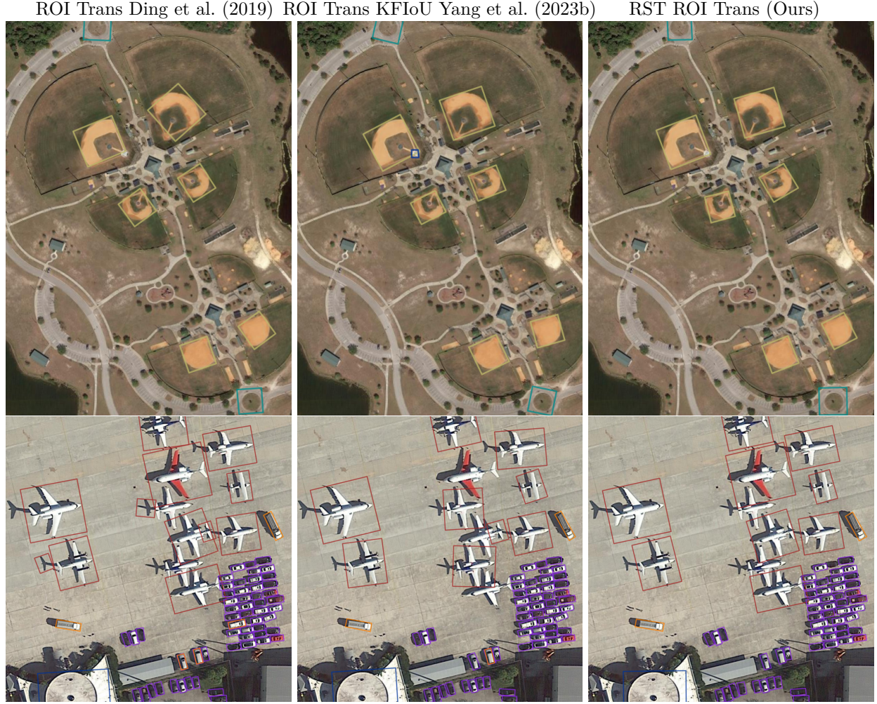
Figure 6: Qualitative comparison between ROI Trans (Ding et al., 2019), ROI Trans KFIOU (Yang et al., 2023b) and the proposed method (RST ROI Trans), on some DOTA examples. As shown, the proposed approach predicts a coherent orientation with respect to the detected objects, while the other methods include more error in their orientation predictions.
