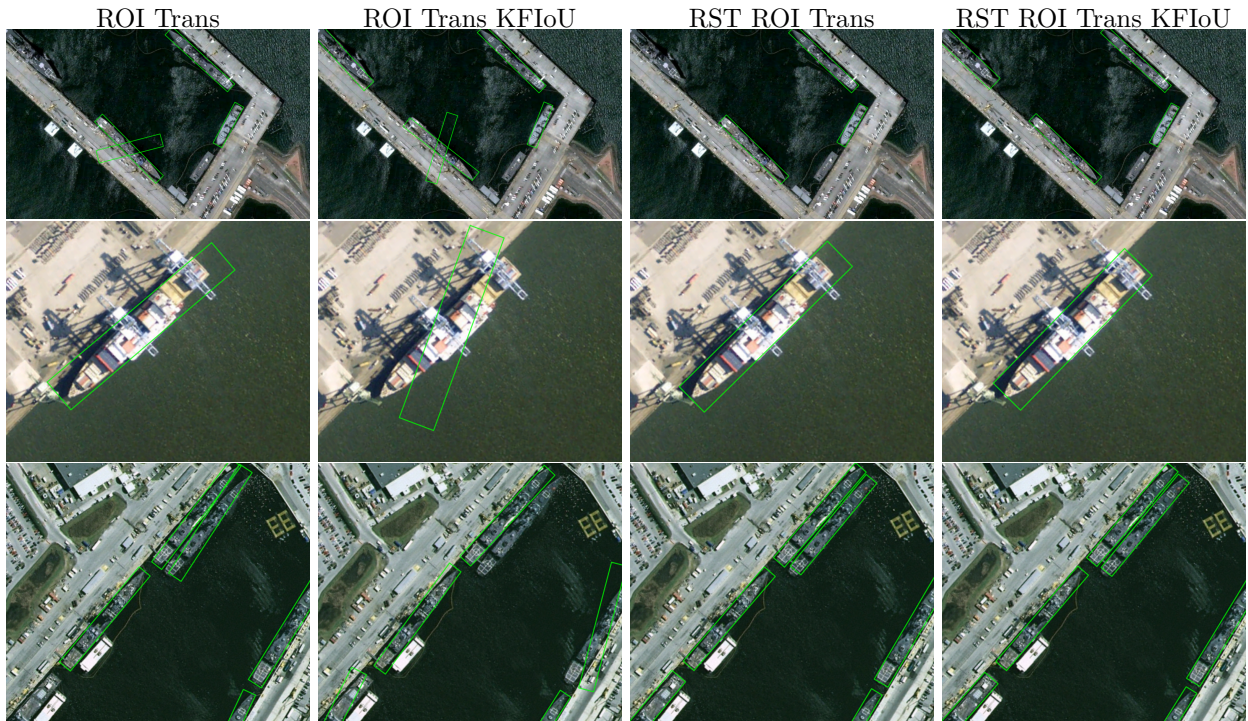
Figure 7: Qualitative comparison between ROI Trans (Ding et al., 2019), ROI Trans KFIoU (Yang et al., 2023b) and the proposed method (RST ROI Trans and RST ROI Trans KFIoU), on HRSC2016 examples. The relaxed structure tensor models achieve considerable improvements with respect to the original methods on angle prediction.
