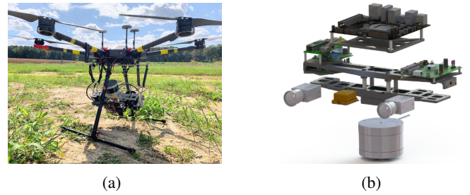
Fig. 1: DJI M600 with sensor payload: (a) isometric view of DJI M600 with sensor payload; (b) Exploded view of sensor payload and key components.
