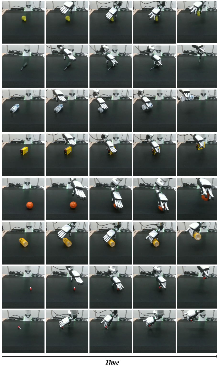
Figure 7: Grasping trajectories from real-world tests. DemoGrasp learns distinct finger poses for large, small, and thin objects to maximize expected success. Slight robot-table contact is leveraged to grasp tiny objects (second-to-last row). A regrasp behavior emerges when an attempt fails (last row).
