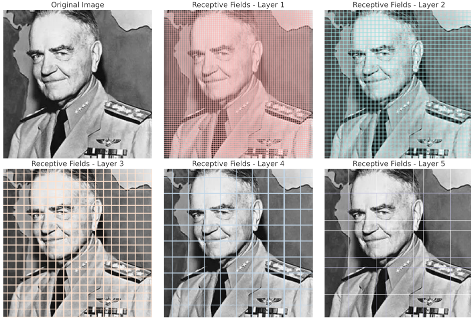
Figure 4: The receptive field size of different CNN layers. Each box represents the effective receptive field.
