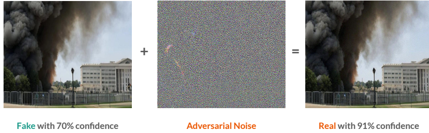
Figure 1: Adversarial attack on the commercially available detector provided by sightengine . Successful evasion is shown by adding adversarial noise computed on the detector by Corvi et al. (2023). We perform an extended evaluation on commercial detectors in Appendix C.
