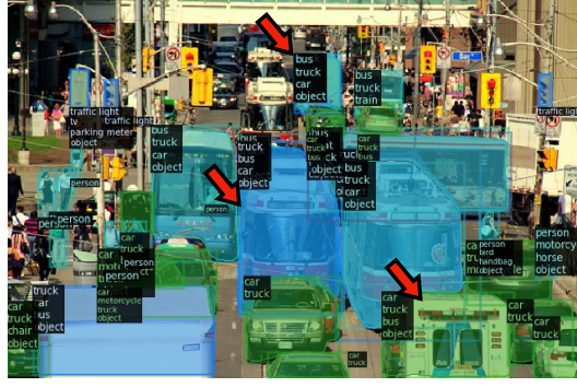
Figure 8: Illustration of the benefits of the proposed RG-PT hyperparameter selection scheme over the state-of-the-art LTT and PT for an object detection application [4]. The red arrows mark the objects not detected by an object recognition model calibrated using LTT or PT that are instead detected by the same model calibrated via RG-PT (see Appendix H.4 for details).
