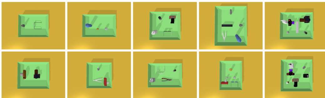
Figure 10: Example configuration of 3D shapes that enables the robot place each object in a given sequence without colliding into other objects already placed. All the bottles, dispensers, and bowls affords only side grasps.
