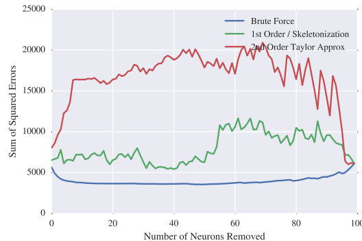
Figure 21: Degradation in squared error after pruning a single-layer network trained to do a one-versus-all classification of the digit 2 using the iterative re-ranking algorithm
