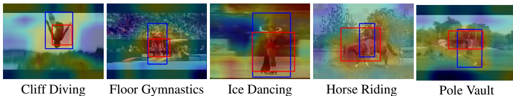
Figure 8: Examples of spatial attention for action localization. (Best viewed in color.) Blue bounding boxes represent ground truth while the red ones are predictions from our learned spatial attention. Our spatial attention mechanism is able to focus on important part of the action, while the ground truth bounding boxes labels focus on the entire human pose. As in the training stage, the ground truth bounding boxes are not used, and the model can only depend on crucial spatial area rather than the entire action to make prediction. For actions with object interactions, such as Horse Riding and Pole Vault , the ground truth box focuses on human pose while the model focuses on objects (such as Horse, Pole) as well.
