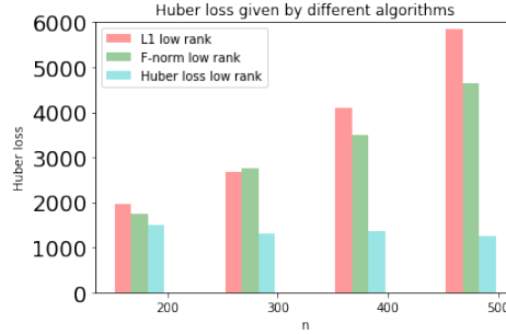
Figure 2: The Huber loss given by different algorithms. The red bar is for the entrywise \ell_1 low rank approximation algorithm [18]. The green bar is for traditional PCA. The blue bar is for our algorithm. For input size n = 200, 300 , all the algorithms output rank-12 approximations. For input size n = 400, 500 , all the algorithms output rank-14 approximations.
