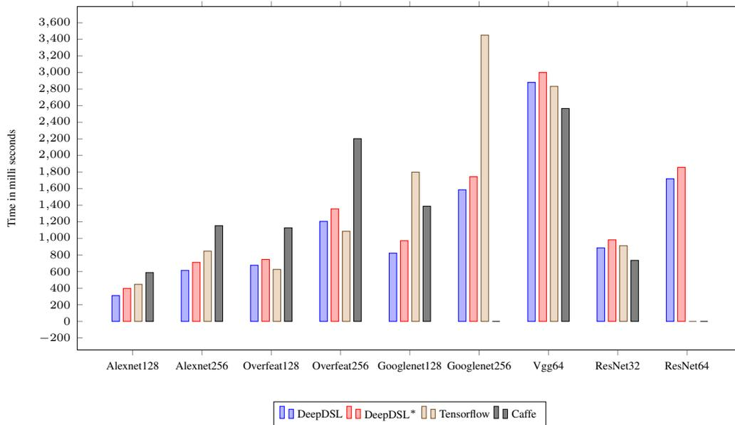
Figure 4: Runtime performance of DeepDSL, Tensorflow, and Caffe (1 forward/backward iteration). DeepDSL and DeepDSL\* are performance in runtime-efficient and memory-efficient mode respectively. The names of the networks are followed by the batch size. Caffe failed to run GoogleNet (batch 256) and ResNet (batch 64) and Tensorflow failed to run ResNet (batch 64) due to exhaustion of GPU memory.
