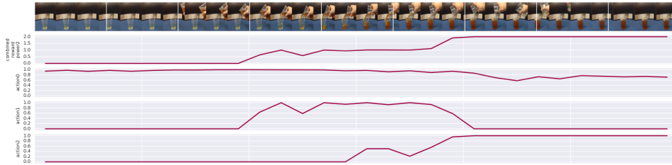
Figure 8: Combining intermediate rewards into a single reward function. From top to bottom, we show the combined reward function (with range [0,2]) followed by the reward function of each individual steps (with range [0,1]). The first step reward corresponds to the initial resting state of the demonstration and is ignored in the reward function. The second step corresponds to the pouring action and the third step corresponds to the glass full of liquid.
