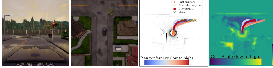
Figure 1: We apply our approach to navigation in CARLA [Dosovitskiy et al., 2017]. Columns 1,2 : Images depicting the current scene. The overhead image depicts a 50\text{ m}^2 area. Column 3 : LIDAR input and goals are provided to our deep imitative trajectory model, and plans to the goals are computed under the model’s likelihood objective, and colored according to their ranking under the objective, with red indicating the best plan. The red square indicates the chosen high-level goal, and the yellow cross indicates a point along our plan used as a setpoint for a proportional controller. The LIDAR map is 100\text{ m}^2 , and each goal is \geq 20\text{ m} away from the vehicle. Column 4 : Our model can incorporate arbitrary test-time costs, and use them to adjust its planning objective and plan ranking.
