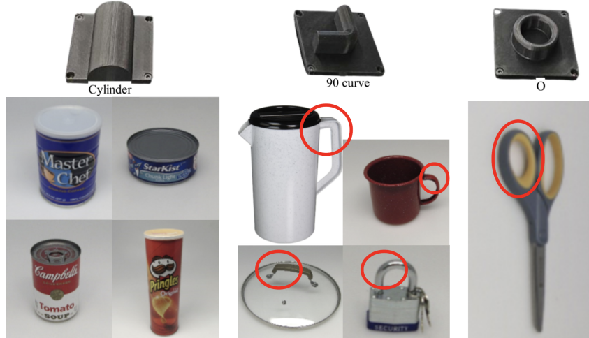
Figure 7: Our 3D-printed objects are analogous to parts of common real-world items. For example, our cylinder resembles the cans from the YCB object set, the 90-degree curve represents the handles on mug and lid as well as locks, and the O-shape is similar to the handle of the YCB scissors.
