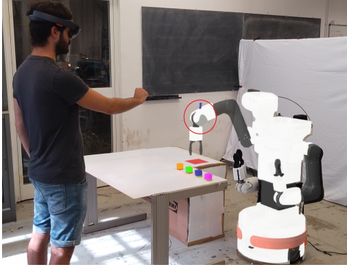
(a) An experimenter conducts a holographic KT session with the Tiago++ robot, teaching actions by manipulating the grey holographic sphere, superimposed on the robot's wrist.
