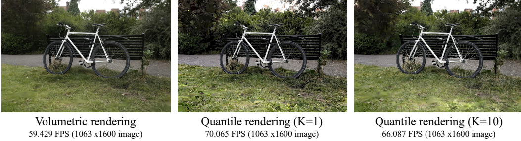
Figure 11: Comparison between V-Render and Q-Render on RGB reconstruction using a pre-trained 3D-GS model without fine-tuning. Q-Render shows only minor PSNR degradation, demonstrating that it serves as an efficient and accurate approximation of V-Render in the RGB domain.
