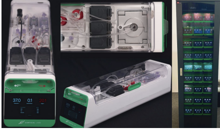
(a) The CL1 biocomputer platform includes an integrated microelectrode array(MEA) and perfusion system for maintaining neuronal cultures. Adapted from [11].
