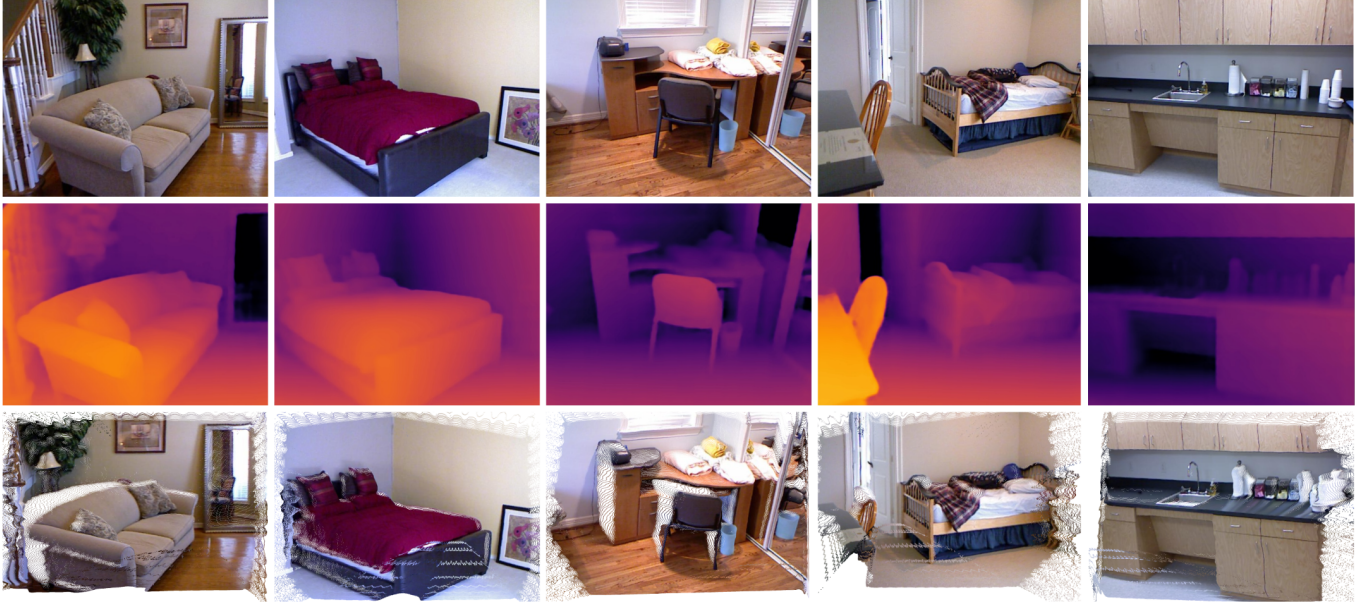
Fig. 1: Our EDADepth model takes single image ( top ) and estimates depth using a pre-trained U-Net model. It uses the BEiT semantic segmentation model to extract context for the generation of depth maps ( Middle ). 3D point cloud ( Bottom ) is constructed from the estimated depth map and the respective input RGB image.
