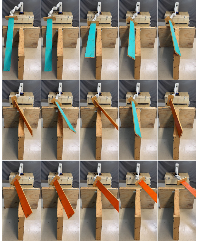
Fig. 1: Kinova Gen3 manipulator transferring and flipping (from blue side to orange side facing up) a long heavy wooden plank across a partitioned space by bracing against the environment for support.
