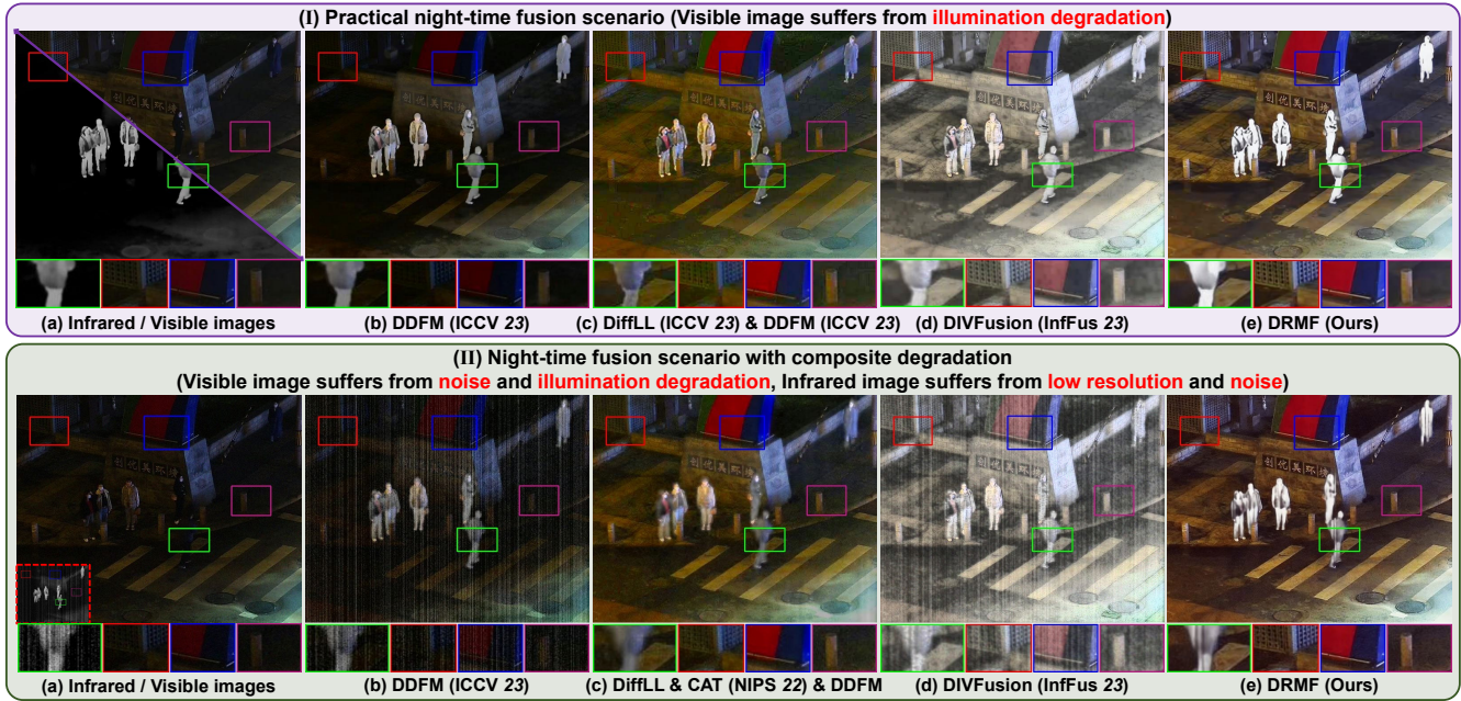
Figure 1: Fusion schematic in challenging scenarios for MMIF tasks. DDFM [64] and DiffLL [12] are Diffusion-based methods for image fusion and low-light image enhancement. DIVFusion [40] is an illumination-robust image fusion method, and CAT [2] is a SOTA universal image restoration method for preparatory denoising and super-resolution.
