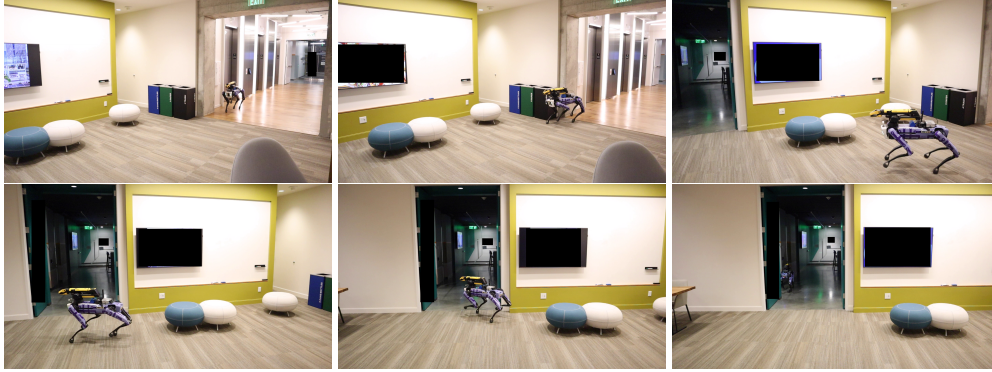
Figure 7: One run of the Spot robot navigating the real-world LAB environment using a kinematically trained policy from AI Habitat. The robot successfully navigates a hallway, moves around furniture and turns into the next hallway before stopping. In contrast, the native BD controllers without a map can only reach visible goals.
