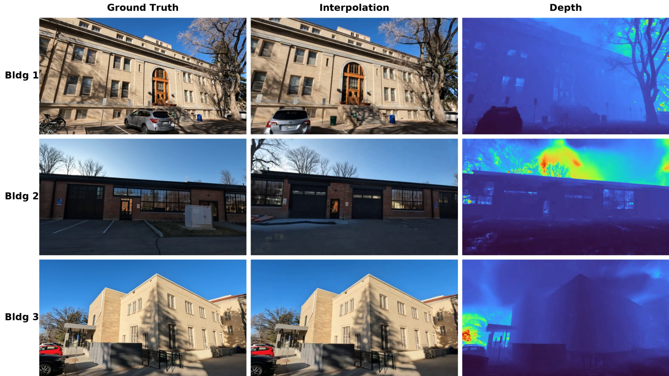
Figure 7. Qualitative results of 3D Gaussian Splatting applied to three campus buildings from the [UNI]101 dataset. Each row shows a different building, with columns displaying (left to right) a ground truth input frame, a novel view synthesized via camera path interpolation, and the corresponding rendered depth map. These results demonstrate that the same video data used for classification and detection naturally extends to 3D reconstruction tasks, supporting a progressive educational curriculum.
