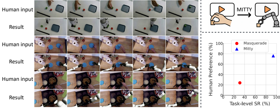
Figure 1: We propose Mitty, a paradoxical in-context learning–based video generation method built on Diffusion Transformers. It can convert human demonstration videos into robotic manipulation videos and achieves high task success rates.
