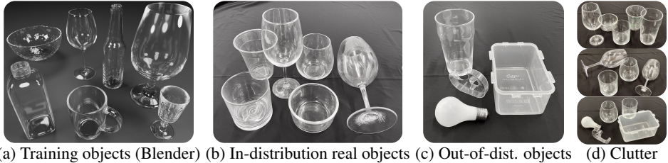
Figure 5: Training and testing objects. (a) shows Blender rendering of the 7 objects we use in data generation for computing grasps and rendering in various stable poses. Objects in (b) are real objects we considered in-distribution with the training objects. We also test on out-of-distribution objects shown in (c). To test grasping in clutter, we setup various testing scenes with objects in and out of distribution, with examples shown in (d).
