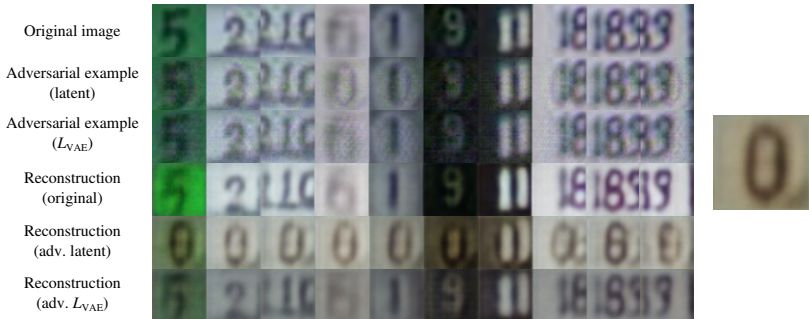
Figure 2: Summary of different attacks on SVHN dataset: original images, adversarial examples for both methods (latent and \mathcal{L}_{VAE} ) and reconstructions of original images and adversarial examples. The \mathcal{L}_{VAE} attack seems ineffective against SVHN in our experiments. Target reconstruction is shown on the right.
