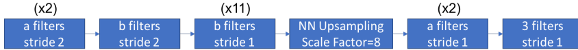
Figure 5: The general architecture of a linear CNN with a filters on upsampled representations and b filters on downsampled representations. We denote the downsampling version of this network as Network D_{a,b} and the non-downsampling version Network ND_{a,b} .
