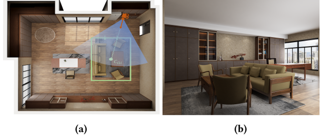
Figure 6: An example of a side view. (a) the camera faces the object group at a slant. (b) the corresponding photograph.
