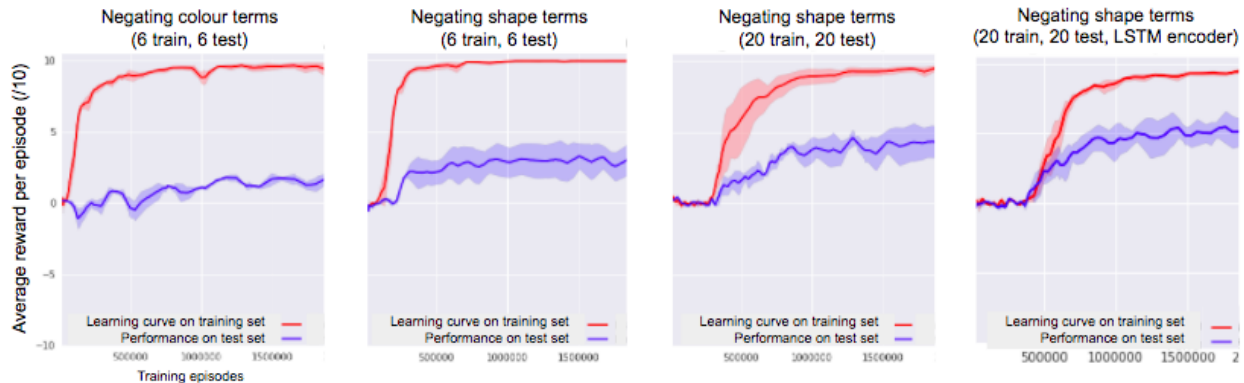
Figure 3: The problem of learning negation in language learning agents: The agent must be exposed to negative instructions in a sufficiently diverse range of contexts in order to learn a useful generalisable notion of negation. If trained to interpret positive commands involving 12 terms and negative commands involving 6 of those 12 terms (left, colour terms, middle, shape terms), the agent does not effectively interpret negative commands involving the remaining 6 terms. When exposed to 40 shape terms and trained to interpret negative commands involving 20 of those terms, the agent generalises the negation operation more effectively, but still not perfectly. When the two-word negative instructions are encoded with an LSTM rather than additive BOW encoder, an almost identical pattern of gradually improving generalisation is observed.
