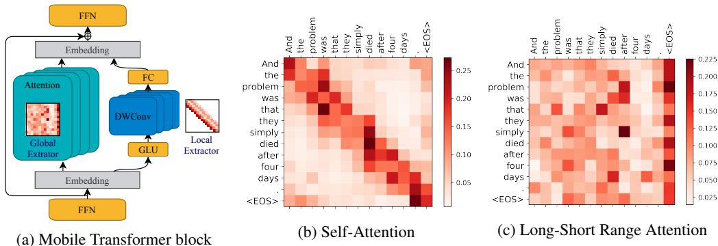
Figure 3: Model architecture (a) and the visualization of attention weights. Conventional attention (b) put too much emphasizes on local relationship modeling (see the diagonal structure). We specialize the local feature extraction by a convolutional branch which efficiently models locality, so that the attention branch can specialize on global feature extraction (c).
