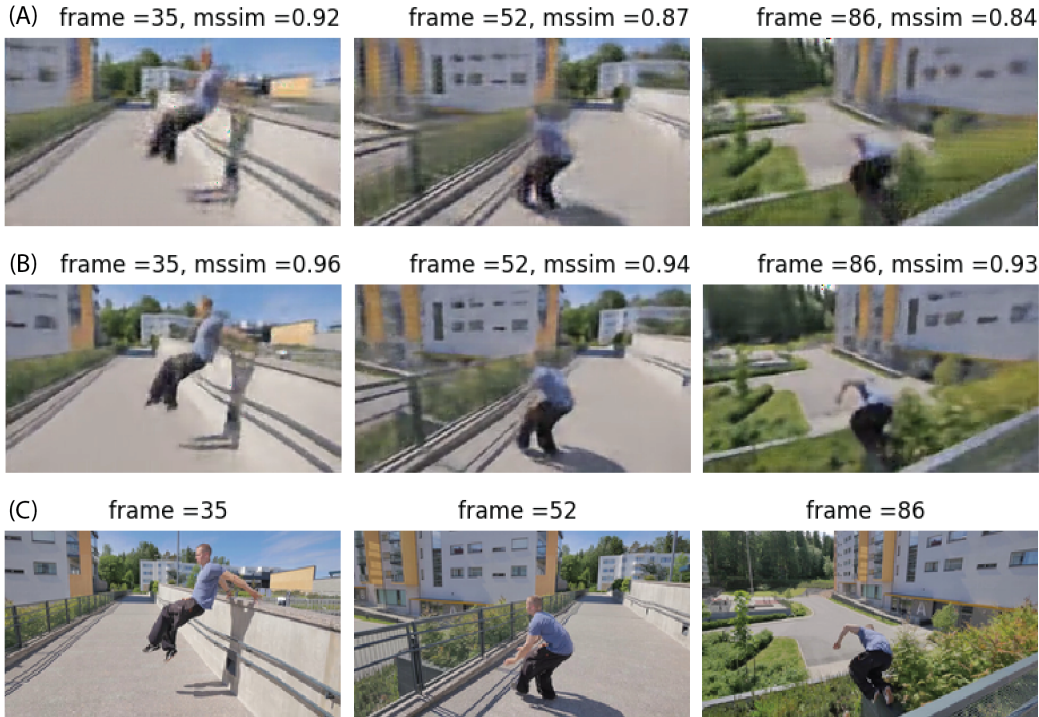
Figure 3: Video encoding reproduction of the DAVIS’ 17 Parkour scene at 120p using the upscaling approach described by eq. 3 with M = 1 . (A) Frames, y_i , produced by the base network f_\theta , with 32 convolution filters per layer, which advances the sequence at each application. (B) Upscaled frames, y_i^* , produced by denoising autoencoder, f_{\theta^*} , with 32 convolution filters per layer. (C) Associated ground truth frames, x_i .
