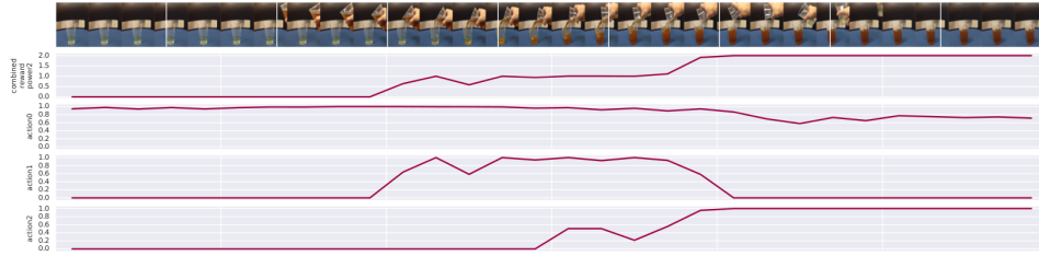
Figure 9: Combining intermediate rewards into a single reward function. From top to bottom, we show the combined reward function (with range [0,2]) followed by the reward function of each individual steps (with range [0,1]). The first step reward corresponds to the initial resting state of the demonstration and is ignored in the reward function. The second step corresponds to the pouring action and the third step corresponds to the glass full of liquid.
