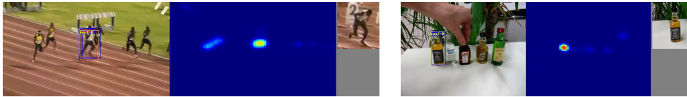
Figure 1: The output of our conditional detector. The two examples show: Left - the detector input. Middle - the heatmap output of our detector depicting the likelihood of the target object centered on each pixel. Right - the “target” template image specifying the object instance to detect.
