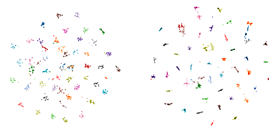
Figure 3: tSNE visualization of the embeddings for 50 classes on Omniglot. The embeddings of unlabeled data got magnetized to the class prototypes forming more compacted clusters in our PRWN right in contrast to the embeddings of PN left
