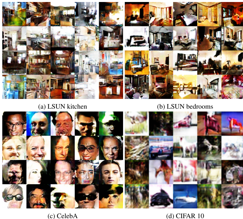
Figure 3: Prior-data-disagreement samples. We visualize samples for which the likelihood under the GAN prior is high, but low under the data-induced prior. Note that most of these samples are of poor visual quality and contain numerous artifacts.
