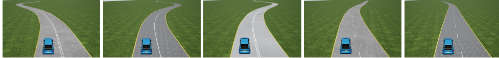
Figure 3: Examples of different road environments randomly generated for each episode in our lane following simulator. We use procedural generation to randomly vary road texture, lane markings and road topology each episode. We train using a forward facing driver-view image as input.
