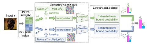
Figure 2: The implementation of Dual Randomized Smoothing (DRS). The image is down-sampled into two non-overlapping sub-images by utilizing two predefined 2x2 pixel indexes.
