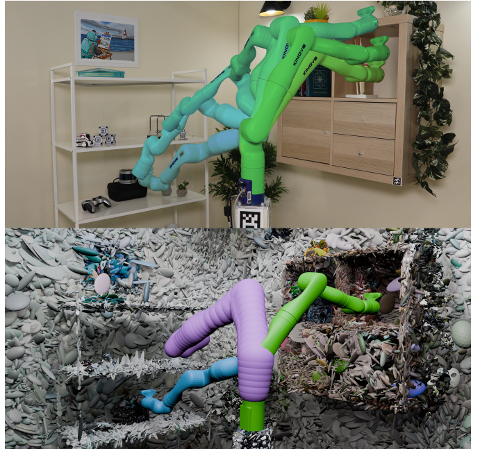
Fig. 1: SPLANNING constructs risk-aware trajectories in a Gaussian Splatting map in real-time. The top image shows a real-world scene that a 7DOF serial manipulator must plan through, starting at the blue configuration (left) and ending at the green configuration (right). The scene is represented as a normalized 3D Gaussian Splat. Then, in real-time, SPLANNING solves an optimization problem that constrains the probability that the robot's forward occupancy (bottom center, purple) collides with the scene.
