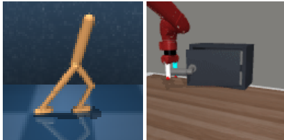
Figure 2: Visualization of our image-based environments. The observations are 64 \times 64 and 128 \times 128 raw pixel images for the walker-walk and sawyer-door tasks respectively. The sawyer-door-close environment used in our generalization experiments in Section 4.2 also uses the same environment as sawyer-door .
