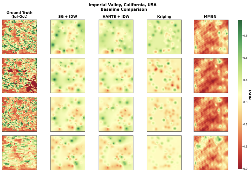
Figure 15: Baseline reconstruction comparison for Imperial Valley, California. Each row corresponds to an equally-spaced temporal frame. The rectilinear irrigation infrastructure creates sharp NDVI boundaries that baseline methods fail to preserve, producing either circular artifacts or smooth gradients. Baseline SSIM values range from 0.0916 to 0.1123.
