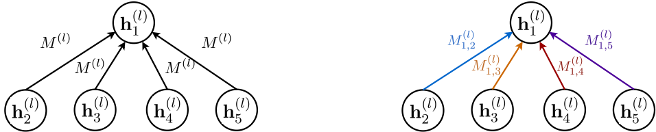
Figure 2: Left. An illustration of the MPNN used in previous flow routing works, which uses the same message function M^{(l)} for aggregating neighbor messages. Right. An illustration of our proposed Per-Edge Weights (PEW), which uses uniquely parametrized per-edge message functions.
