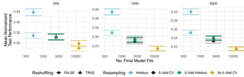
Figure 6: Trade-off between the final number of model fits required by different resamplings and the final average normalized test performance (AUC ROC) after running random search for a budget of 500 hyperparameter configurations. Averaged over different tasks, learning algorithms and replications separately for increasing n (train-validation sizes, columns). Shaded areas represent standard errors.
