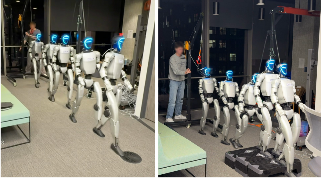
Figure 9: Evaluation of policies at multiple stages. Due to the multi-stage nature of our pipeline, we evaluate the performance on real at multiple stages before going out into the real world. Left: trying our MoCap Pre-Trained policy. Right: Trying the first generalist in a lab environment tracking a pre-defined root trajectory.
