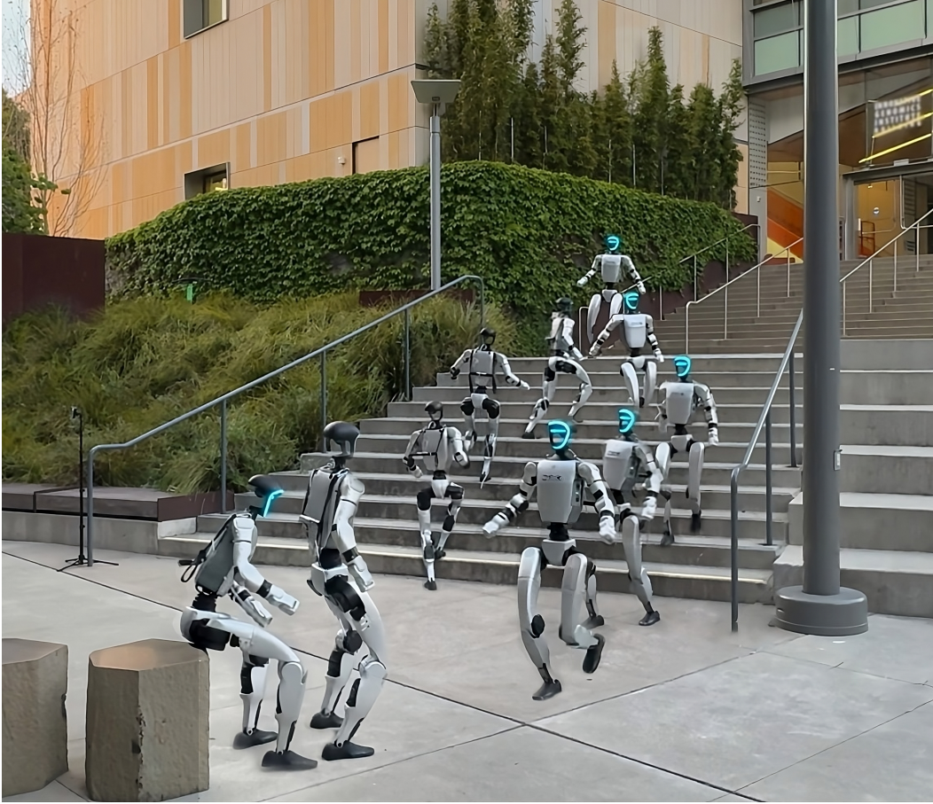
Figure 1: VIDEOMIMIC is a real-to-sim-to-real pipeline that converts monocular videos into transferable humanoid skills, letting robots learn context-aware behaviors (terrain-traversing, stairs-climbing, sitting) in a single policy. Video results are available on our webpage: https://videomimic.net .
