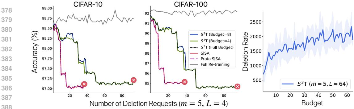
Figure 6: (Left) We report the impact on performance of S<sup>3</sup>T and baselines with an increasing number of deletion requests. S<sup>3</sup>T handles a higher number of deletion requests while maintaining high performance with a relatively low budget (⊗ indicates the failure point for the system). (Right) We report the deletion rate of S<sup>3</sup>T with an increasing budget and observe steady growth.
