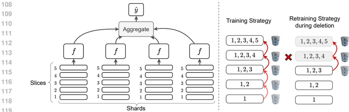
Figure 1: Schematic diagram of the Sharded, Isolated, Sliced, and Aggregated training (SISA) (Bourtole et al., 2021) framework. An ensemble of models is individually trained on disjoint shards. (Left) Each shard is further divided into slices. (Right) Each model is sequentially trained on the slices and checkpoints are stored. After deletion, retraining resumes from the best available checkpoint.
