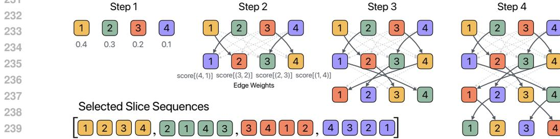
Figure 4: Illustration of the BMS algorithm. BMS selects one element for each permutation at a time. This is done by constructing a bipartite graph with all feasible edges to the next node, where edge weights are the current sequence scores. We compute the maximum weight matching on this graph. The dark gray arrows ( $\rightarrow$ ) indicate the selected edges and dotted arrows ( $\dashrightarrow$ ) the feasible ones.
