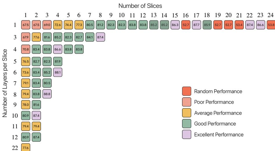
Figure 11: Performance impact of S<sup>3</sup>T when allocated a different number of layers per slice: We observe that simply increasing the number of slices can lead to a significant performance drop. There is an optimal tradeoff between the total number of slices and the number of layers per slice.
