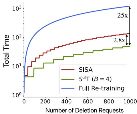
Figure 15: We compare the deletion time as the number of deletion requests increases. S<sup>3</sup>T requires the lowest deletion time compared to SISA and full re-training.
