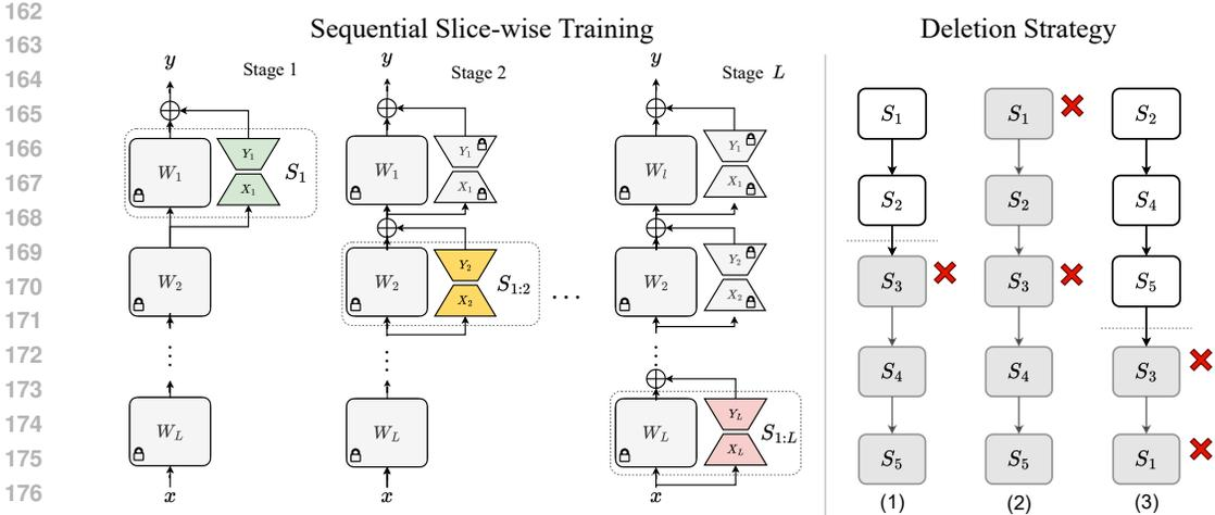
Figure 2: (Left) We show the schematic diagram of the slice-wise training strategy in  $S^3T$ . We incrementally train the model –  $i^{\text{th}}$  layer (from the top) using slices  $S_{1:i}$  while keeping the other layers fixed. (Right) We show the impact of deletion on models trained on different permutations of slices.
