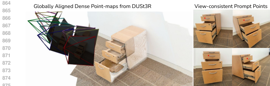
Figure 9: 3D part segmentation from Pose-free RGB images. Illustration of how DUST3R (Wang et al., 2023b) is used to achieve 3D part segmentation from unstructured RGB images. For each object, we take around 10 pose-free RGB images as input to the pre-trained DUST3R (Wang et al., 2023b) model, which outputs a set of globally-aligned 2D-to-3D dense point-maps, i.e., every 2D pixel on each image is matched to a point in 3D. This correspondence enables cross-view pixel matching via finding nearest-neighbor in 3D space. We can therefore sample view-consistent 2D points for prompting our fine-tuned SAM model, and the resulting segmented masks are grouped into 3D part segmentation.
