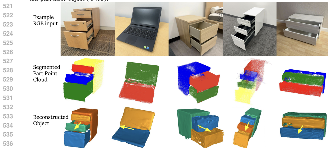
537 Figure 7: We evaluate Real2Code on real world objects using RGB data. For each object, we use 10 pose-free 538 RGB images captured in-the-wild and run Real2Code with DUST3R(Wang et al., 2023b). We show one example 539 RGB input (1st row), segmented point clouds (2nd row) and full reconstruction (3rd row) for each object.
