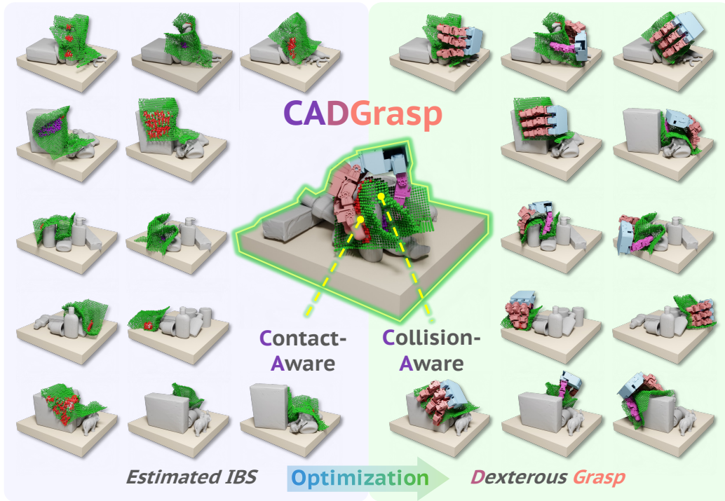
Figure 1: We propose CADGrasp , which learns a contact- and collision-aware intermediate representation as a constraint, and further obtains the dexterous grasp pose with an optimization method to achieve single-view dexterous hand grasping in cluttered scenes.
