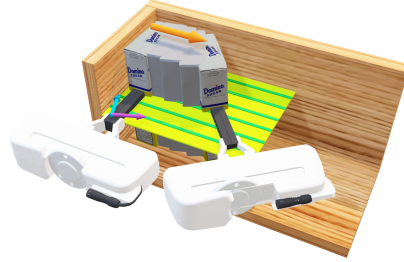
Figure 3: HFVC execution with partial information with example pivoting motion (start pose is object on the left). Gray objects represent linearly interpolated object poses used by proprioception-based object pose estimation. Object translation is exaggerated for visual clarity. Blue arrow represents direction of force command, purple is velocity. Velocity commands are projected onto the (green) plane containing the interpolated end-effector trajectory.
