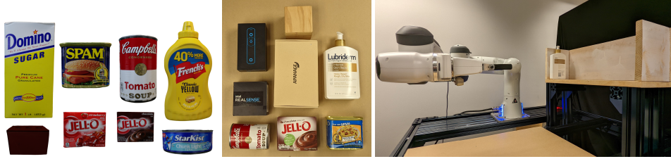
Figure 4: Object-in-Shelf Task Domain. Left: cuboid and cylindrical YCB objects used in simulation for training the HFVC precondition. Middle: objects used in real-world experiments. Right: real-world setup.
