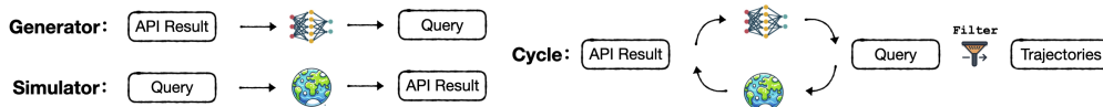
Figure 1: The Generator can leverage the LLM to create potential user queries based on the available API information. The Simulator can interact with the environment using these queries to achieve API response results. The cycle consistency constraint between them can extract high-quality synthetic execution trajectories in the absence of explicit human supervision.
