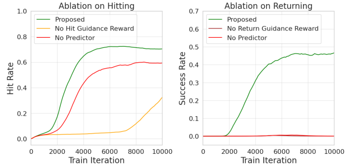
Fig. 5. Ablation study of the key components of the proposed framework based on training results. Including both the predictor in the actor policy and prediction-based reward designs prove to be crucial for learning successful strikes. Note that the metrics during training are lower than those during testing shown in Table II. This is due to more frequent environment resets during training for efficient exploration; the immediate post-reset stabilization during training generally leads to missing the first serve.
